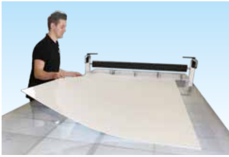
1. Place the substrate on the table.
