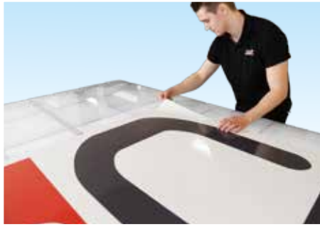
2. Place your adhesive material on top of the receiving material.
