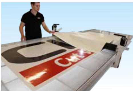
4. Pull the adhesive material halfway over the roller.
