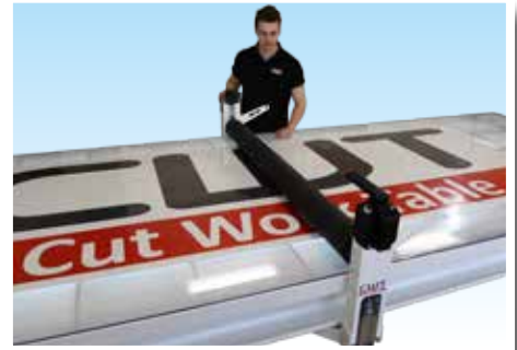
3. Lower the roller for fixation.
