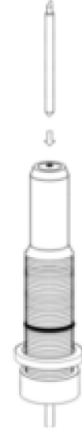
STEP 4: Carefully insert the blade into the top of the blade holder
